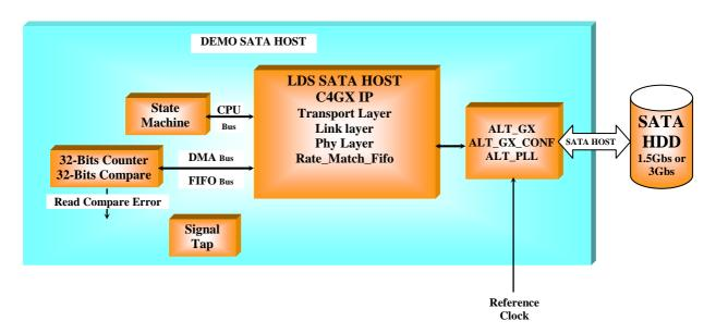
At reset the State machine is doing a disk performance test. The result of the test and several signals can be observed from Signal Tap.
